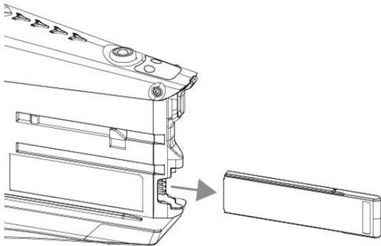
2. Insert the DJI CINESSD into the DJI CINESSD Reader, then connect the DJI CINESSD Reader\* to a computer.
